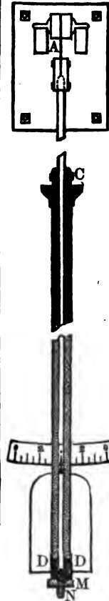
Fig. 2.—Section of high, with a dome-shaped top, and twelve Great Westminster pendulum. As it is a 2-seconds pendulum, its centre of oscillation is 13 feet from the top A, which is higher than usual above the centre of gravity of the bob, on account of the great weight of the compensation tubes. The whole weighs very nearly 700lb, and is probably the heaviest pendulum in the world.
